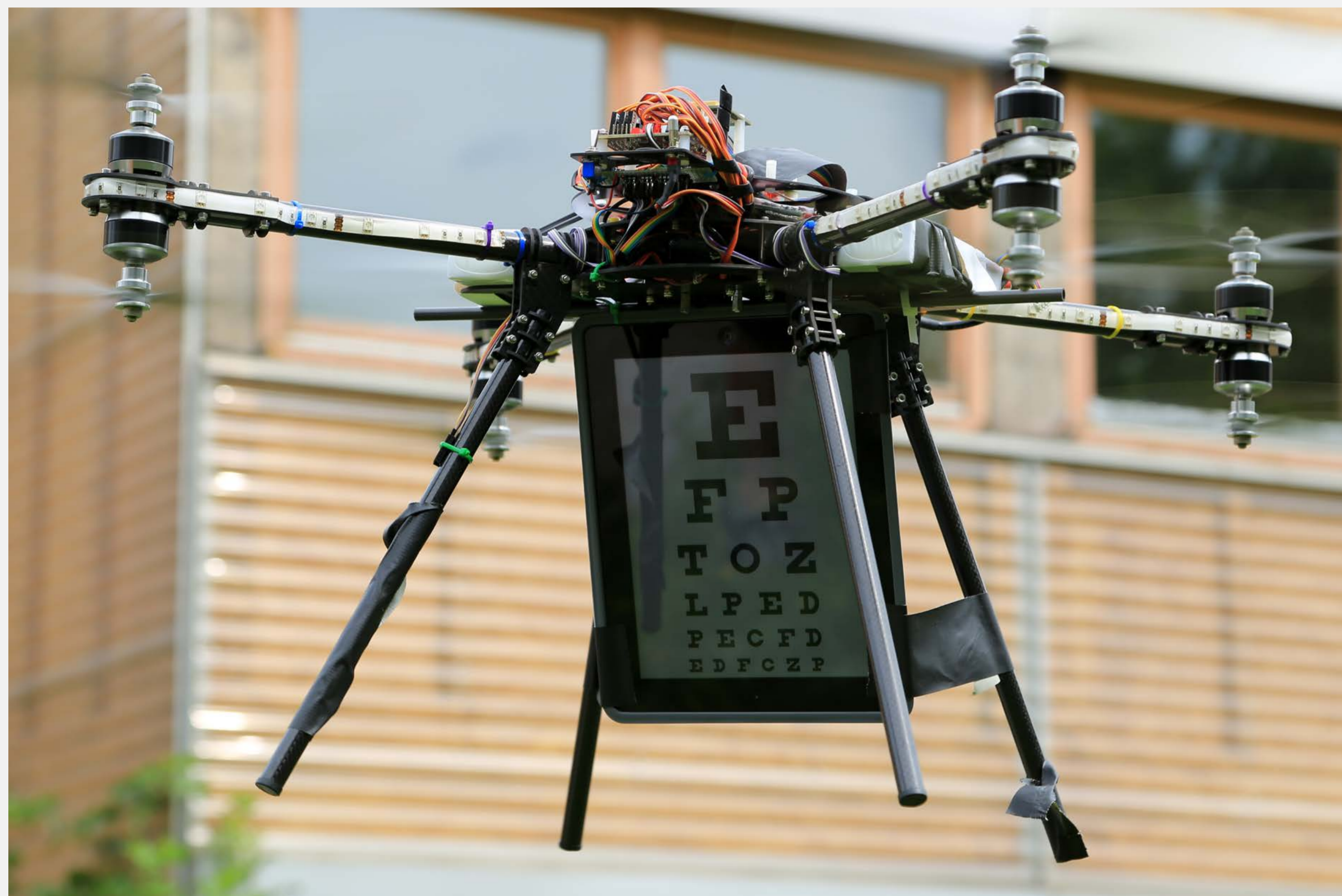
Prototype of the mid-air display: An iPad attached to an octocopter with 8 rotors
