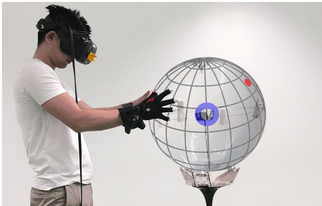
Figure 1: We present TangibleSphere – a setup that allows physical, interactive displays (in our case a spherical display with a diameter of 60 cm) to be simulated inexpensively in VR. We preserve the advantages of such displays’ physical counterparts by enabling tangible interaction, such as free rotation in all directions. Comparing TangibleSphere to a purely virtual display, we found that allowing true physical rotation significantly improves accuracy and reduces task completion time.
