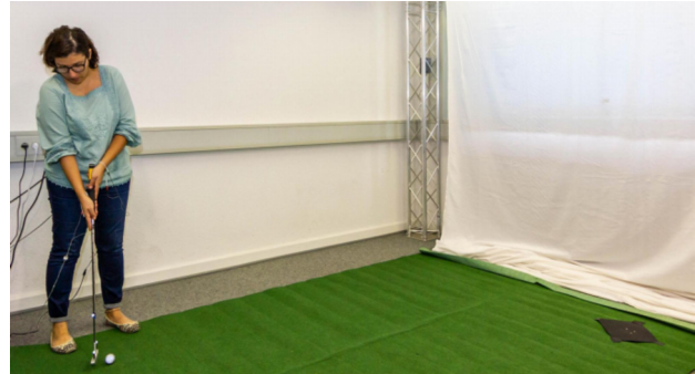
Figure 1: A user testing GeniePutt in a mini-golf scenario. The EMS system supports the user by turning the wrist so that the club faces the target.
