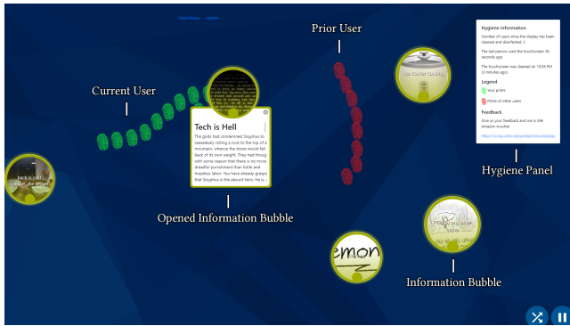
Figure 3: An overview of the hygiene concept and the existing public display application on top of which it was implemented. The hygiene concept displays a panel on the right side, providing hygiene information and explaining the touch traces. Touching the display produces a trace on the screen. For the current user, the traces are green, and for past users, the traces are red.
