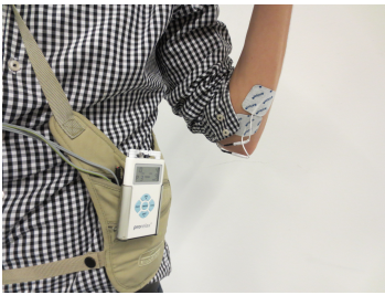
Figure 2: An EMS feedback system: A user wearing a mobile EMS feedback system that is attached to the forearm.
