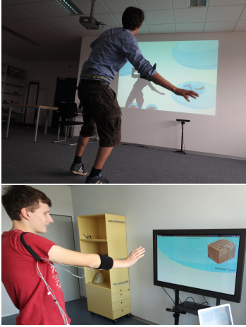
Figure 1: Free-hand interaction with haptic feedback: A user receives haptic feedback when approaching an object on the screen.
