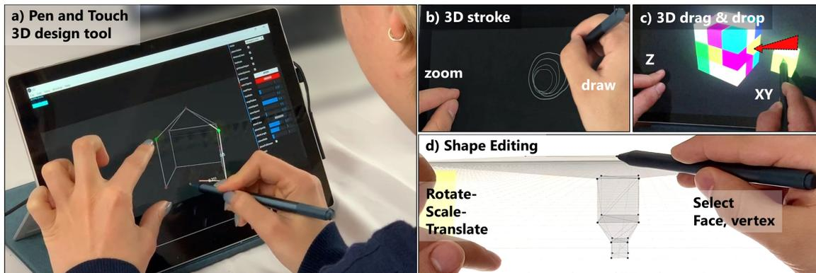
**Figure 1:** *Bi-3D* is an interaction concept to create and manipulate 3D objects and sketches. E.g., to edit shape points (a), draw a 3D stroke (b), 3D drag & drop an object (c), or scale shape (d) – enabled by a dynamic coupling of pen and touch in both hands.
