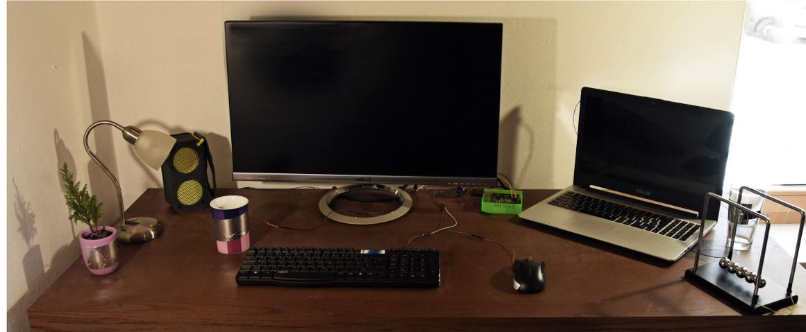
**Figure 1:** Desk setup with *Interact2Authenticate*: We integrated our prototype (in a green, 3D printed case) to a desk setup for a preliminary usability study. The setup is based on our findings from Table 1.
