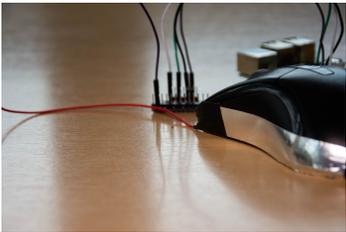
**Figure 3:** Workaround: Adding additional foil to non-conducting surfaces to recognise touch input by means of capacitive sensors.
