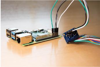
**Figure 2:** *Interact2Authenticate* prototype: A Raspberry Pi connected to capacitive touch sensors.
